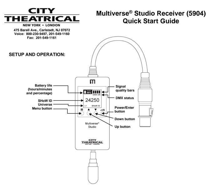
**Multiverse**<sup>®</sup> **Studio Receiver 900MHz/2.4GHz** can be set up as a receiver in a multi universe system with a Multiverse Transmitter, or in a single universe system with a Multiverse Node or Multiverse SHoW Baby.
